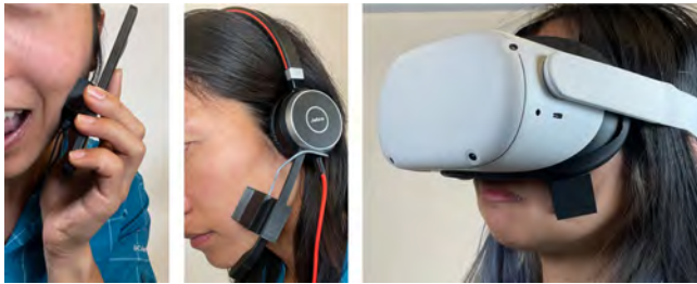
Figure 13: Mock-ups of Füpöp electronics integrated into a cell phone, an audio headset, and a head-mounted display.
